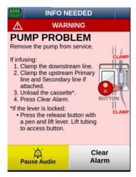
• If this failure occurs during an active infusion and flow is interrupted, this could lead to an underdose. (See Image 2 below)
